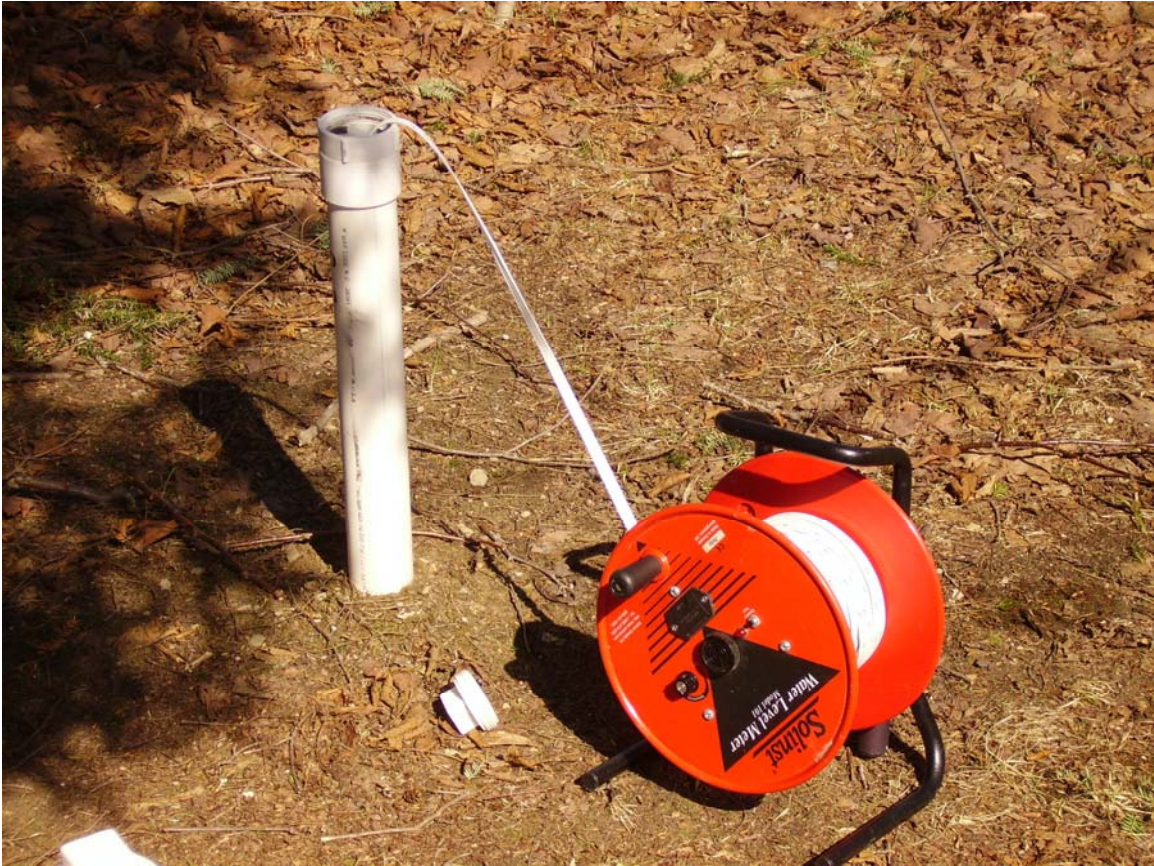
Figure 5. Solinst Water Level Meter in use at B1
